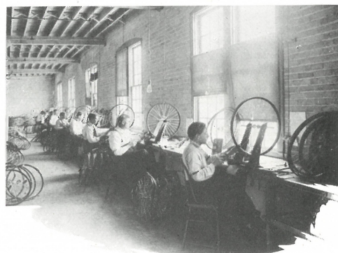
The skill which comes with long experience is needed for the fine operations of wheel truing
